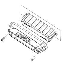
③ Install the LED module on the mounting surface by 2 screws
