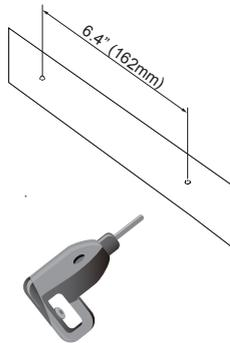
② Drill 2 holes on the mounting surface "
