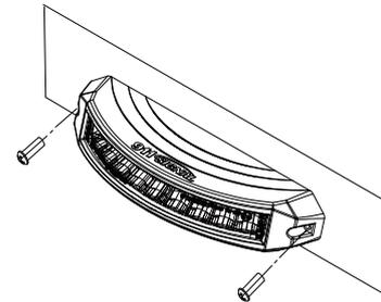
③ Install the LED module on the mounting surface by 2 screws
